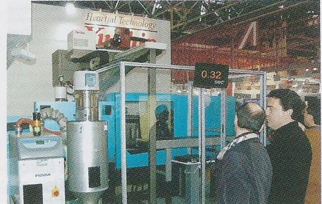
Yushin: Robot takes the part out at a zippy 0.32 second.
