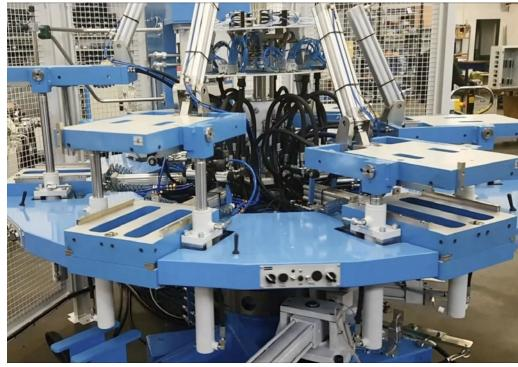
tary presses is equipped with a frequency converter of the main electric motor, representing an energy saving solution with electric energy saving of 15 - 45%, depending on the production cycle.
